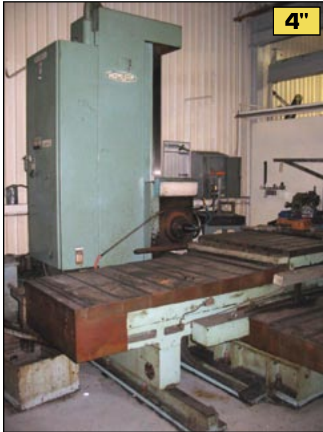
Nomura Horizontal Boring Mill
