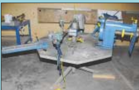
Elbow Edge Fabrication Fixture
