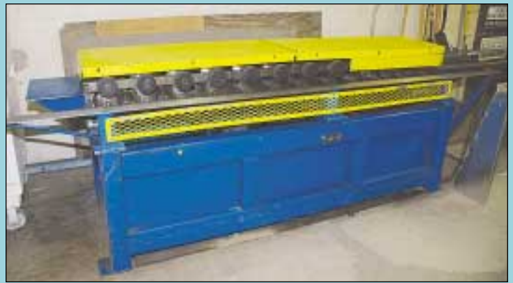
(7) Duct Roll Forming Machines By TDC, Lockformer and Engel
