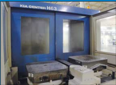
Kia Model H63 Two-Pallet CNC HMC w/ 24" Pallets and No. 50 Spindle
