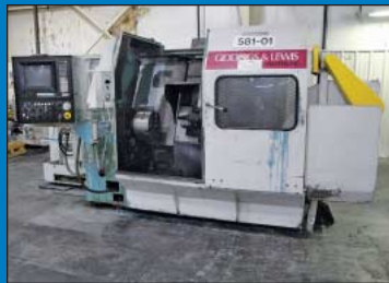
Giddings and Lewis Model Masterline 40C CNC Turning Center w/15" Chuck
