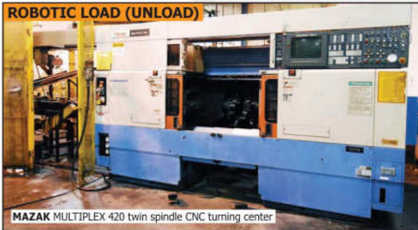
MAZAK MULTIPLEX 620 twin spindle CNC turning center
