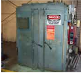
Controlled Pyrolysis Cleaning Furnace
