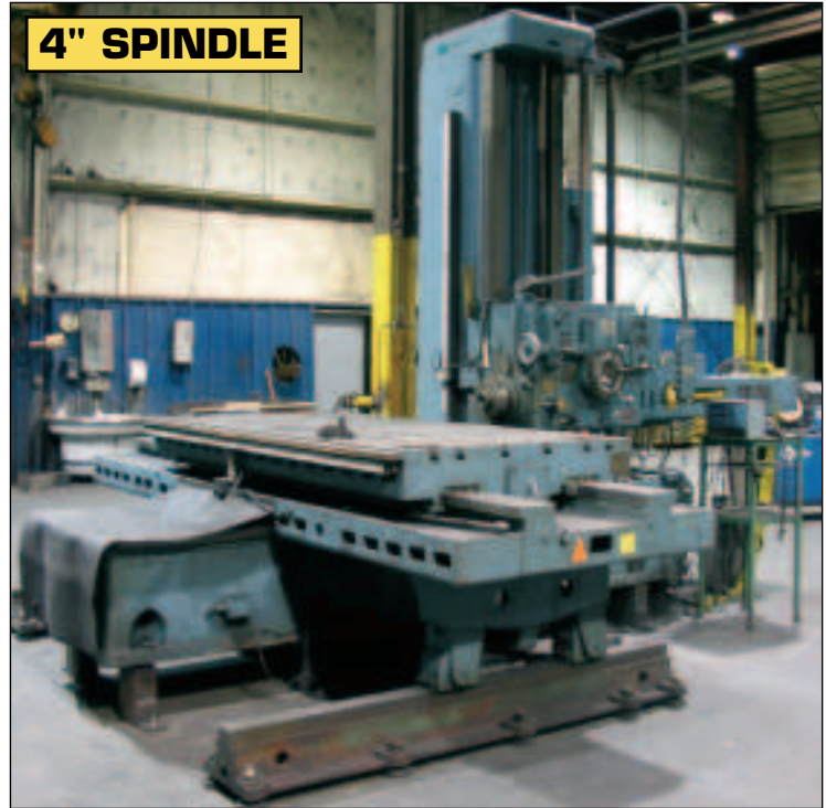
G & L Hybormill Horizontal Boring Mill
