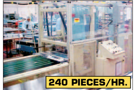
T-Drape Footer Sheeter and Hot Melt Applicator
