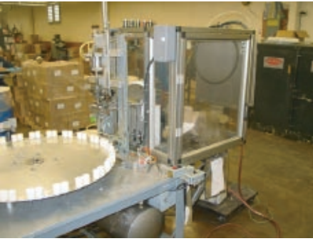
Cozzoli 2-Head Piston Filler with 24-Station Rotary Indexing Table Complete With Diving Nozzles, Approx 22ft Long X 10in Wide Rubber Belt Pack Off Conveyor
