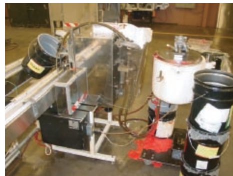
Kenwell Twin Piston Fillers (2) With Auto Indexing, Diving Nozzles, Puck Conveyor System, S/S Hot Pot, Swanmatic Manual Chuck Capper (Serial # C-300-3336 With Speed Controller, Cherry Burrell S/S Piston Metering Pump (Serial # 20187 With S/S Cone Hopper And S/S Cover, S/S Conveyor With Dc Variable Speed Drive With Rubber Belting, (2) S/S 4 Pass Serpentine Cooling Stations With Witt Model MMA070 300 Psi Compressors
