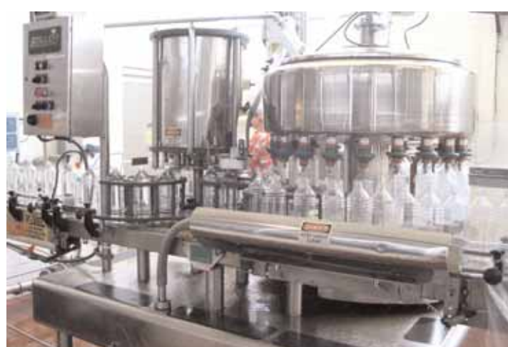
Filler Specialties 21-Head Rotary Filler & Cap Sorter & Feeder
