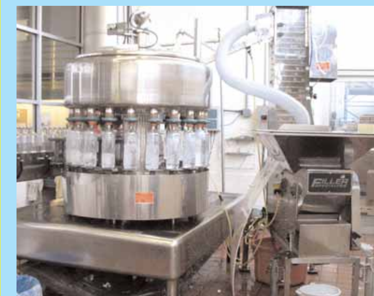
Filler Specialties 21-Head Filler, Capper & Feeder -Palmerton, PA
