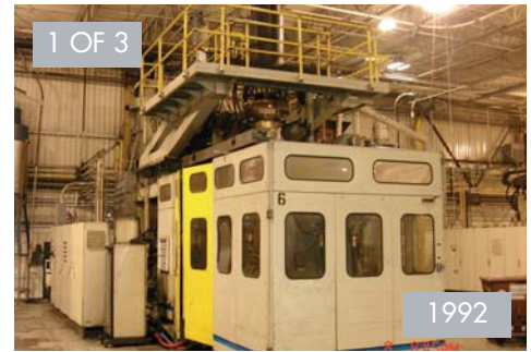
MORETTI/UNILOY MODEL MORETTI M-400 SINGLE HEAD DUAL-SCREW BLOW MOLDING MACHINE
