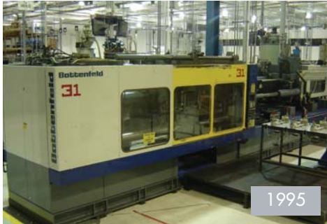
BATTENFELD 750 TON INJECTION MOLDING MACHINE
