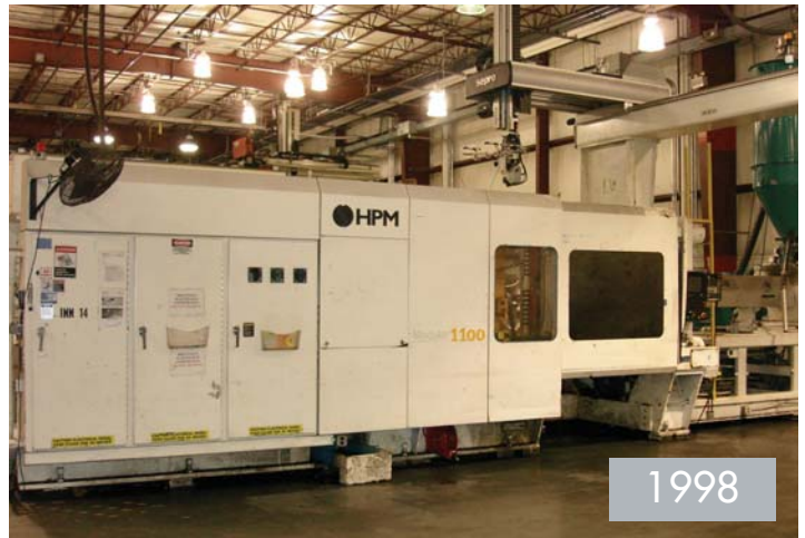
HPM MODEL MLH1100WP-160 1,100-TON INJECTION MOLDING MACHINE
