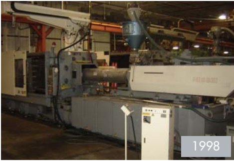
1998 NISSEI FN 9000 620-TON INJECTION MOLDER
