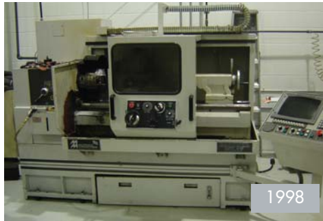
MILLTRONICS MODEL PARTNER ML17 17" X 36" CNC LATHE
