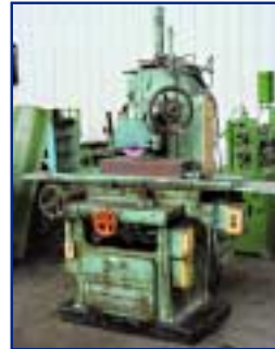
8" X 24" GALLMEYER & LIVINGSTON HYDRAULIC SURFACE GRINDER
