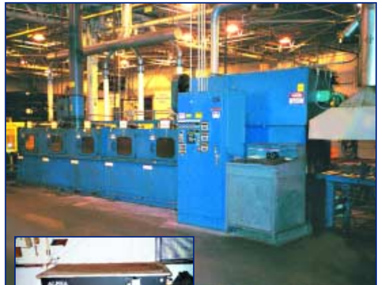
MAGNUS 5-STAGE PARTS WASHER W/ ALPHA OIL SEPARATION SYSTEM
