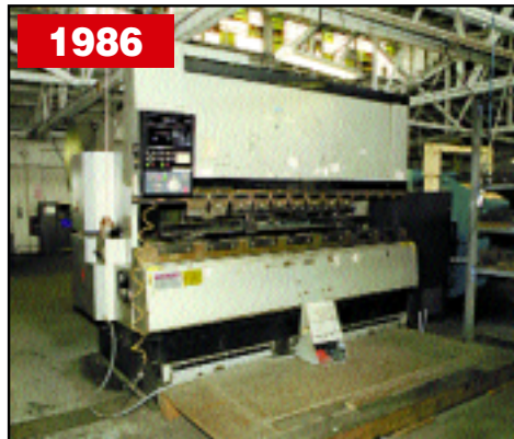
150-TON X 10' AMADA HYDRAULIC, MDL. FBD-1503
