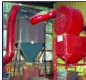
AAF PULSE DUST COLLECTOR
