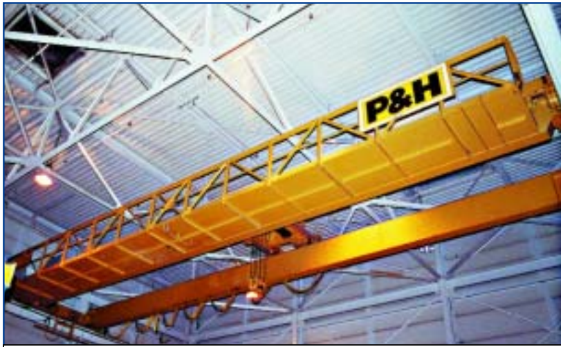
10-T P&H Overhead Bridge Crane
