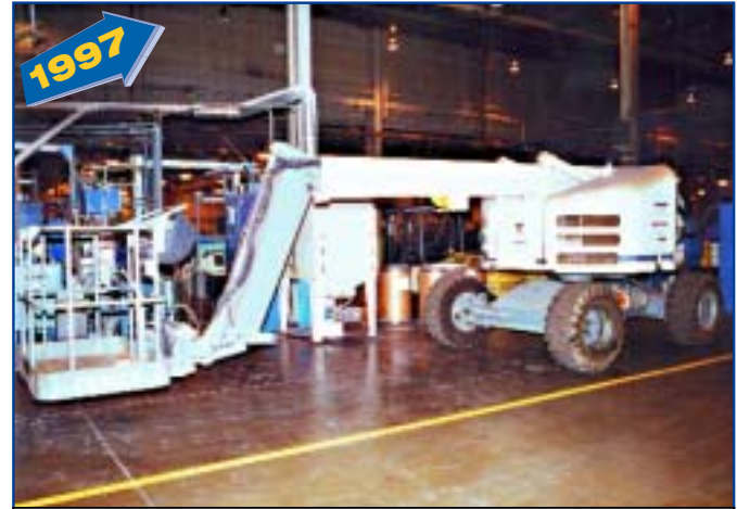
500 Lb. HI-JACK/TEREX Man Lift, Mdl. TA64
