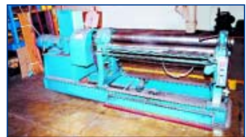
ROLSHEAR, INC. Initial Pinch Type Plate Bending Roll, Mdl. 2C
