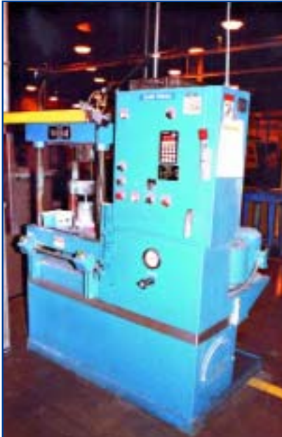
50-T WABASH Up-Moving Hydraulic Sample Press, Mdl. #V50-15-X
