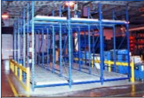
40"x30"x24' 9-Zone Gravity Powered Retrieval System
