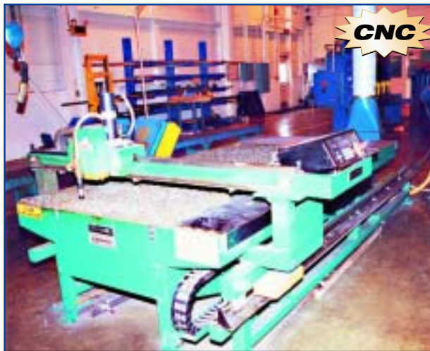
LOCKFORMER VULCAN CNC Single Torch Plasma Shape Cutter
