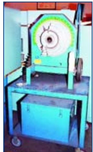
GREENLEE Electric Pipe Bender, Mdl. 555
