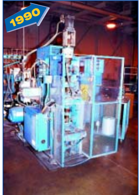
30-Ton KUX Powder Metal Press, Mdl. 60B
