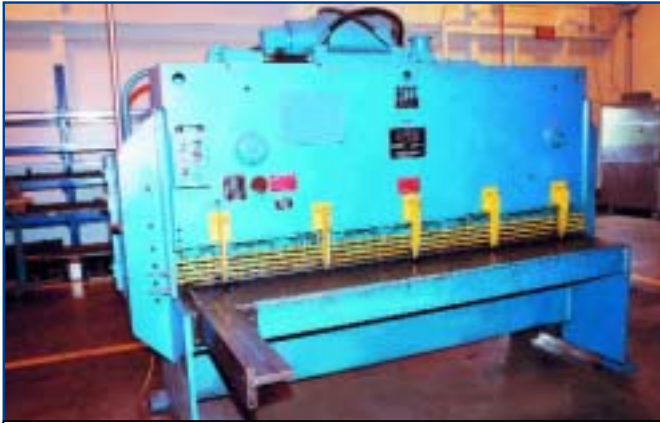
HTC Hydratool Power Squaring Shear, Mdl. 250-8A
