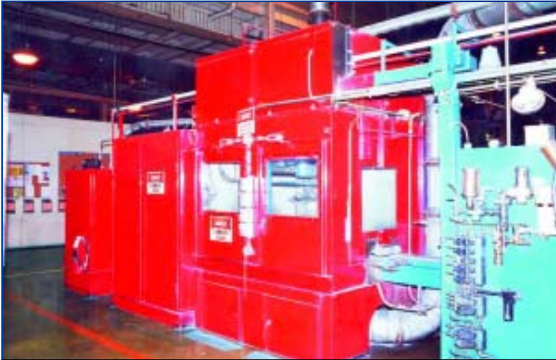
BINKS Spray Type Alcohol Degreaser
