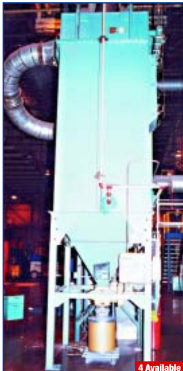
4'x4'x8' FLEX KLEEN #100WSBS-49 Air Pulse Dust Collector
