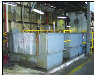
4' X 8' X 3' HEAT TECH, HEATED DIP TANKS
