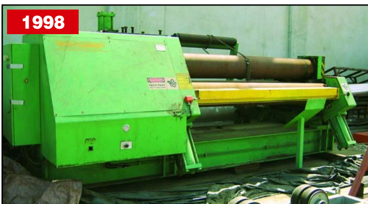
10' X 1" CAPACITY J.M. MONTGOMERY HYDRAULIC PLATE BENDING ROLL, MDL. 4R-120100
