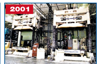
BATTENFELD / KRAUSS - MAFFEI RETROFITTED DUAL PRESS RIM MOLDING SYSTEM, (2) BATTENFELD 4-POST HYDRAULIC DOWN ACTING PRESSES, MDL. WF
