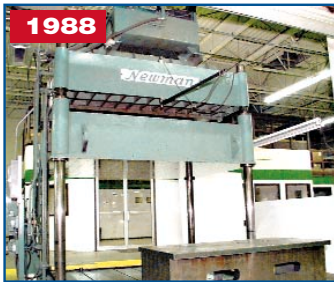
1988 NEWMAN 250-TON CAPACITY 4-POST HYDRAULIC DOWN ACTING DIE TRYOUT PRESS
