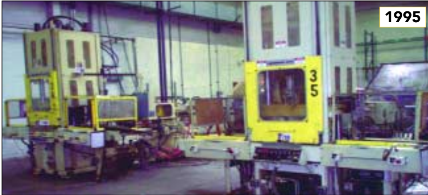
1995 & 1994 200-TON NEWBURY VERTICAL SHUTTLE
