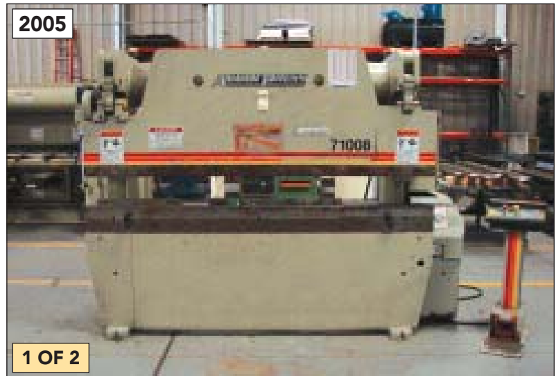
ACCUPRESS 8' X 100 Ton Press Brake
