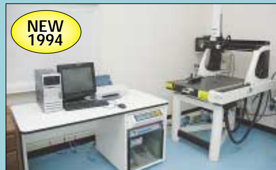
DEA Swift Model RWA001103 Coordinate Measuring Machine
