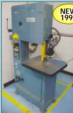
18" Enco Vertical Band Saw
