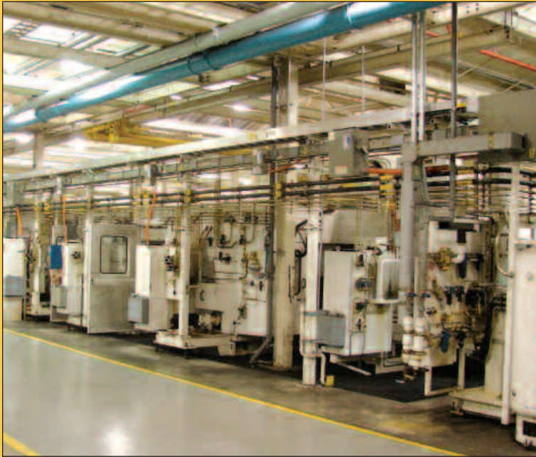
LAMB/NAVISTAR 6.0L & 6.4L POWER STROKE DIESEL V-8 ENGINE CRANKCASE MACHINING PRODUCTION LINE
