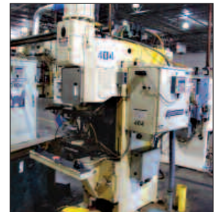
TAYLOR-WINFIELD 100-KVA PROJECTION SPOT WELDER
