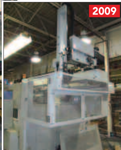
OVERHEAD GANTRY HANDLER FOR OKUMA & HOWA 2SP-35H
