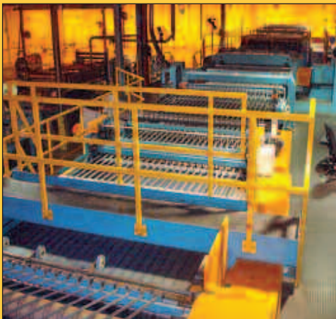
82" PASABAN KDD-2200 FOLIO SYNCHRONOUS ROTARY SHEETER MFG 1999
