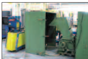
RAPID GRANULATOR W/SOUND ENCLOSURE & FOREMOST GRANULATOR
