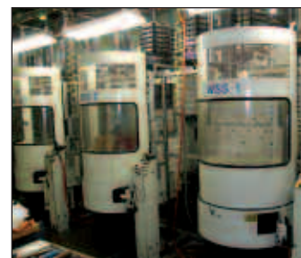
(3) PALLET LOADING & UNLOADING STATIONS FOR MAKINO CELL
