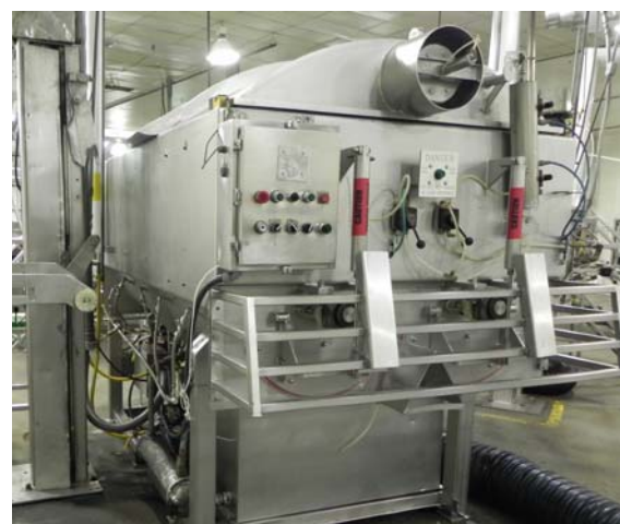
AMFEC 2,000 lb. capacity Sani-Mix Vacuum Mixer/Blender
