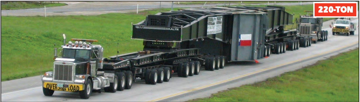
KALYN SIEBERT 220-TON, 25 AXLE HEAVY TRANSPORT TRAILER (SEE WEB SITE FOR DETAILS)
