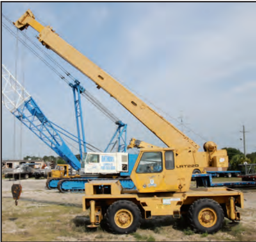
KOEHRING LORAIN LRT-220, 44,000-LB. ROUGH TERRAIN CRANE
