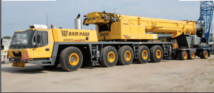
2005 GROVE GMK5240, 240-TON TRUCK CRANE
