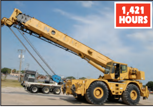
GROVE RT865B, 65-TON, ROUGH TERRAIN CRANE
