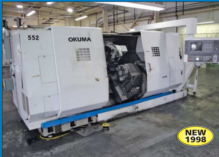
Okuma Model LU-25 Twin Turret Four-Axis CNC Turning Center w/ 47" Centers
