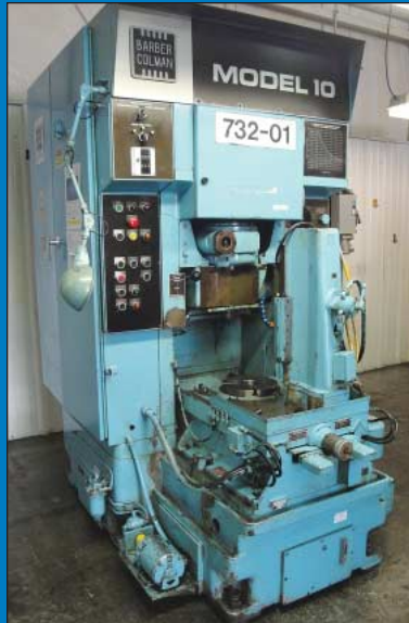
Barber Colman Model 10VGS Vertical Gear Shaper
