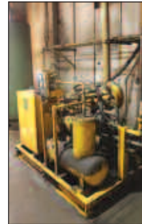
60 HP JOY TWIST WATER COOLED AIR COMPRESSOR
