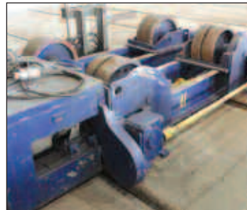
30 TON PANDJIRIS RUBBER COVERED ROLL TANK TURNING ROLLS DRIVE SHAFTS, 20" DIAMETER WHEEL X 10" WIDTH
