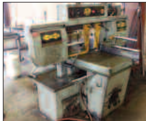
S20 SERIES II HYDMECH HORIZ. BAND SAW
