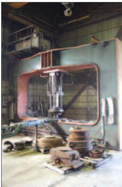
300 TON X 15' O'CONNOR HEAD DISHING AND FLANGE PRESS
