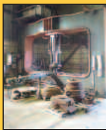
O'CONNOR HEAD DISHING AND FLANGE PRESS
