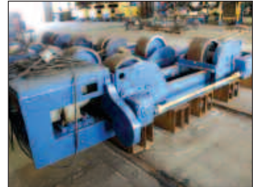
30 TON IRCO RUBBER COVERED ROLL TANK TURNING ROLL
