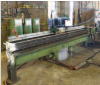
OCONNER 10' SUBMERGED ARC SEAM WELDER
