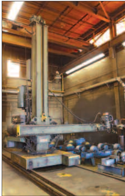
16' X 16' #1600 RBM PANDJIRIS WELDING MANIPULATOR
