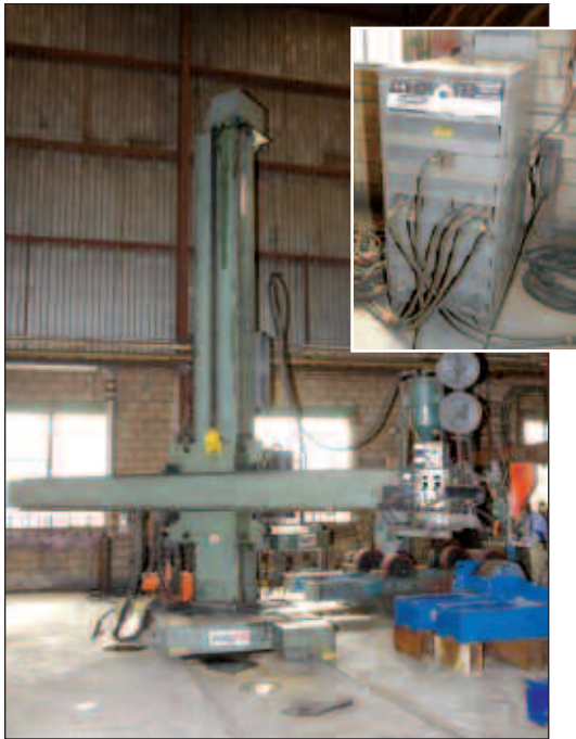
PANDJIRIS #600 16' X 16' TRACK MOUNTED ROTATING WELDING MANIPULATOR
