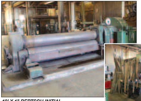
10' X 1" BERTSCH INITIAL PLATE BENDING ROLL
