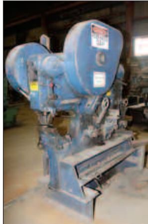
6" X 6" X 1/2" PEDDINGHAUS #210A-20 MECHANICAL IRONWORKER
