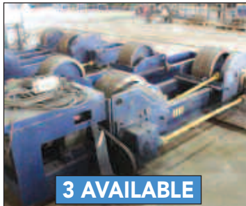
30 TON PANDJIRIS RUBBER COVERED ROLL TANK TURNING ROLLS DRIVE SHAFTS, 20" DIAMETER WHEEL X 10" WIDTH
