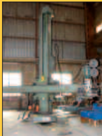
PANDJIRIS #600 16' X 16' TRACK MOUNTED ROTATING WELDING MANIPULATOR
