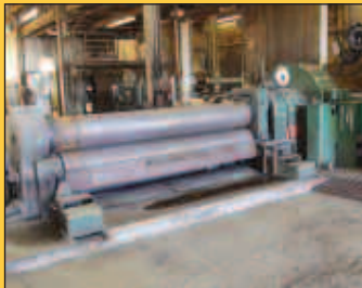
10' X 1" BERTSCH INITIAL PLATE BENDING ROLL
