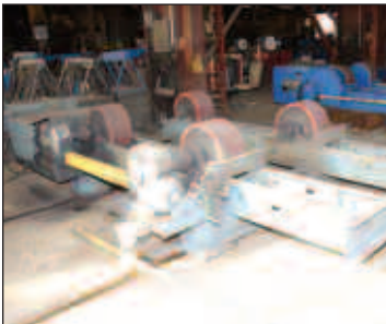
30 TON PANDJIRIS RUBBER COVERED ROLL TANK TURNING ROLLS DRIVE SHAFTS, 20" DIAMETER WHEEL X 10" WIDTH
