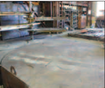
20 TON X 12' IRCO #TT20K 12 ROTARY TABLE WITH WELDING PLATFORM
