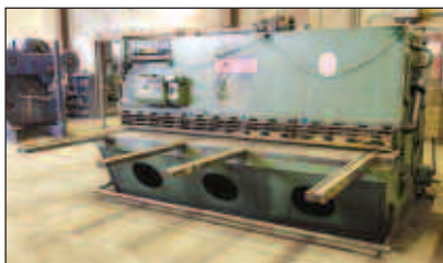
10' X 1/2" PEARSON HYDRAULIC POWER SQUARING SHEAR
