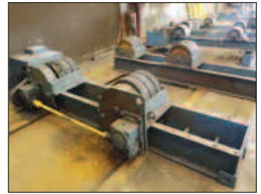
40 TON PANDJIRIS RUBBER COVERED TANK TURNING ROLL
