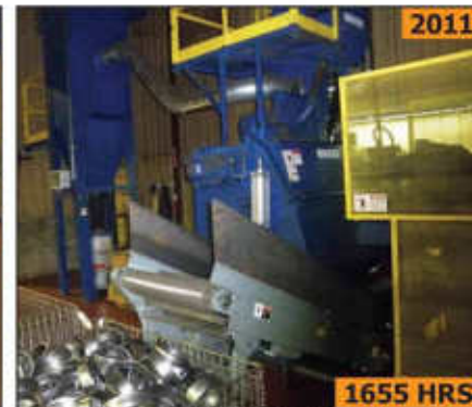
WHEELABRATOR TMS-7-1-25 abrasive shot blast with dust collector (SOLD BY PHOTO ONLY)
