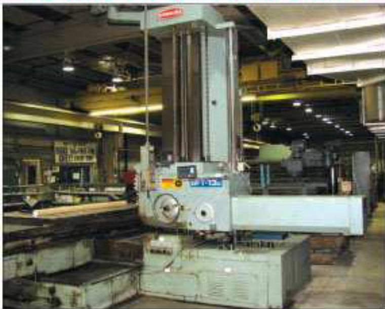
5" SHIBURA MDL. BFT-13C TABLE TYPE HORIZONTAL BORING MILL , Mdl. BFT13CW2PD, S/N 153360, 5.12" Spindle Diameter, 70.9" Vertical Travel, 47" X 98" Table, Spindle Taper #50, 35.4" Spindle Travel, 98.4" Cross Travel, Longitudinal Travel 51.2", Spindle Speeds (27) 9-1200 Rpm, Main Motor 25 Hp, Facing Head, 4-Way Bed, Power Draw Bar, Digital Readouts
