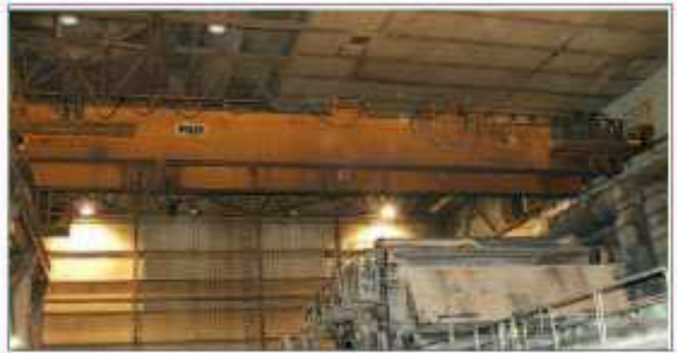
(2) 50 TON 25/25/25 TRIPLE HOIST OVERHEAD BRIDGE CRANES, S/N C27136 & C27137, Total Crane Cap. 50 Ton, Cap. Each Trolley 25 Ton, Span 79'10", Lift Each Trolley 60', 5 Step Variable Speed Control, #105 Magnetorque Braking, Independent End Truck Drive, Radio Controlled
