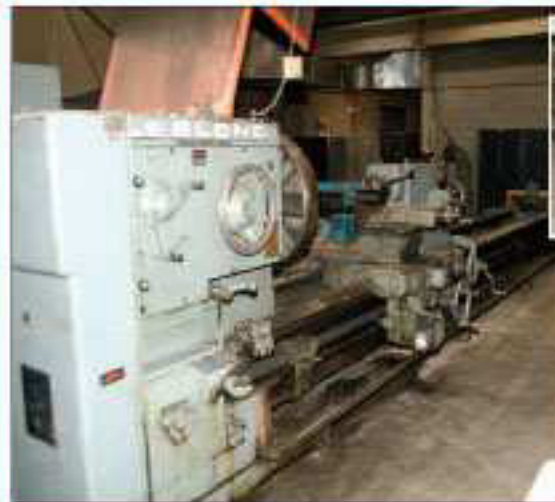
40" X 20' LEBLOND HEAVY DUTY ENGINE LATHE, S/N 3NK962, Rpm 500-600, 40" Swing Over Bed, 20" CC, Equipped w/Taper Attachment, Motorized Rapid, Lead Screw, Thread Dial, Steady Rest, 32" 4-Jaw Chuck, 20" Centers, 3" Spindle Hole
