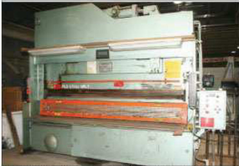
10' X 1/2" & 10' X 1/4" COMBO HYDRAULIC SHEAR & PRESS BRAKE , Mdl. 1505B10, S/N 54078810C41-4, Shear Cap. 10' x 1/2", Brake Cap. 10' x 1/4", 36" Back Gauges, (Manufactured by Elk River Co. Elk River, MN)
