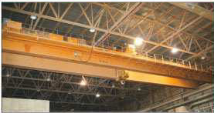
(2) 50 TON P&H OVERHEAD BRIDGE CRANES, S/N C27138 & C27139, Cap. 50 Ton, 102' 10" Span, Lift 60', Welded Box Girder, Static Stepless, #146 Magnetorque Braking, Independent End Truck Drive, Radio Controlled
