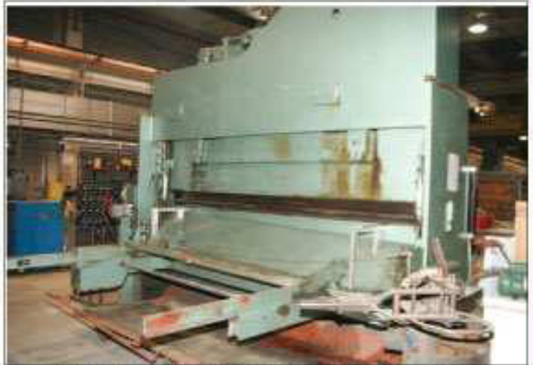
10' X 1/2" & 10' X 1/4" COMBO HYDRAULIC SHEAR & PRESS BRAKE , Mdl. 1505B10, S/N 54078810C41-4, Shear Cap. 10' x 1/2", Brake Cap. 10' x 1/4", 36" Back Gauges, (Manufactured by Elk River Co. Elk River, MN)
