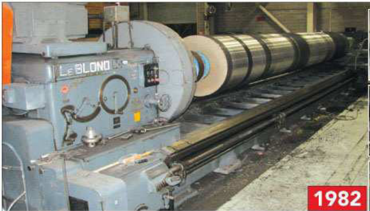
6642 X 474" LEBLOND WIDE BED ENGINE LATHE, S/N RWB546, 7-230 Rpm, 48" Face Plate Type Chuck, Face Plate Drive, Taper Attachment, Full Length Lead Screw, Thread Dial (Late Delivery)
