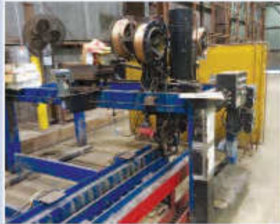
Frame Line Gantry Kentex Sub Cure Dual Head Lincoln, (2) each DC 1000 w/Lincoln NA-3N Feeders, 100' l x 8'
