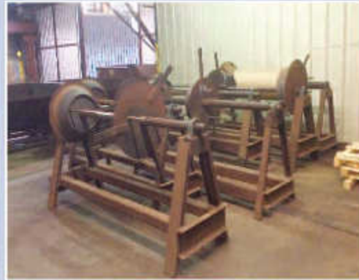
PBR Panel Roll Former Line, American 10,000 lb Decoiler, Upender 48" Coil Length, 14 Stands, Bradbury Roll Former, Flying Shear, Auto Material Stacker
