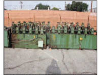
27 Stand x 48" x 3 1/2" Bradbury Rafted Rollformer
