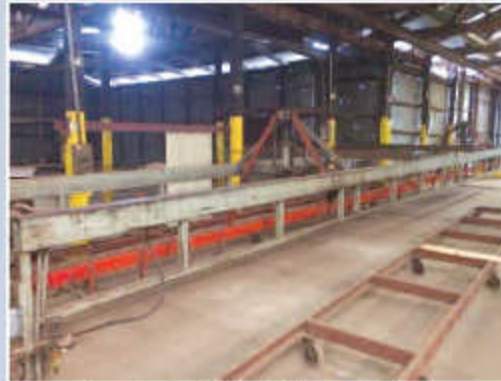
PBR Panel Roll Former Line, American 10,000 lb Decoiler, Upender 48" Coil Length, 14 Stands, Bradbury Roll Former, Flying Shear, Auto Material Stacker
