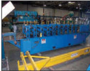
12 Stand x 30" x 2" Bradbury Rollformer
