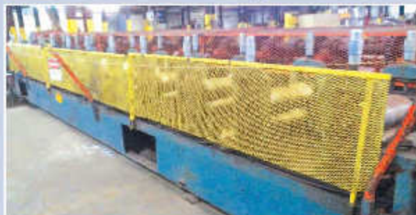
Purlin Roll Former Line, Jamco Decoiler, Strainer, HTC Shear, Omega Roll Former, # Stands 12
