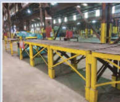
Piranah Mdl. P120 Ton Hyd Iron Worker w/HD In/Out Feed Roller Tables
