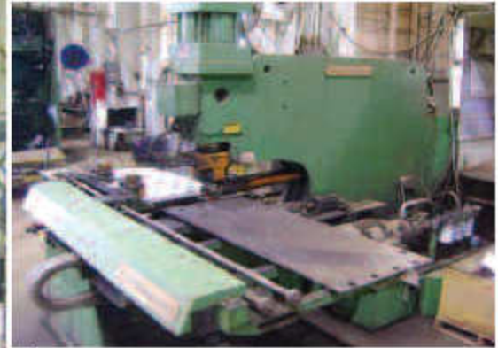
1990 PEDDINGHAUS Mdl. F-1154 30-Ton, S/N C-172, 30-Ton CNC Fabrication Center, Material Size 30" x 120" w/3-Position Fixed Tooling & Fagor CNC Controls
