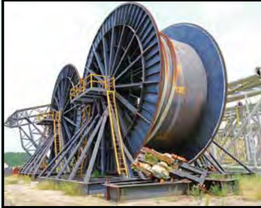
OFFSHORE PIPE LAY REELS
