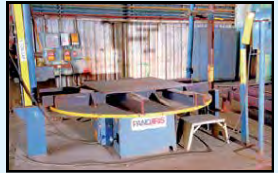
PANDJIRIS MDL. MT200-12VS, 20,000 LB. CAP. WELDING TURNTABLE
