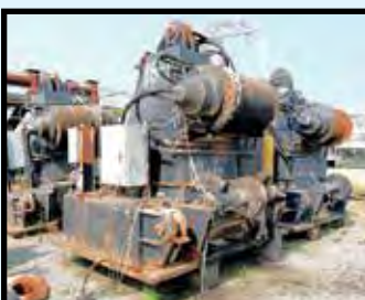
DAVIT SYSTEM HOIST UNITS
