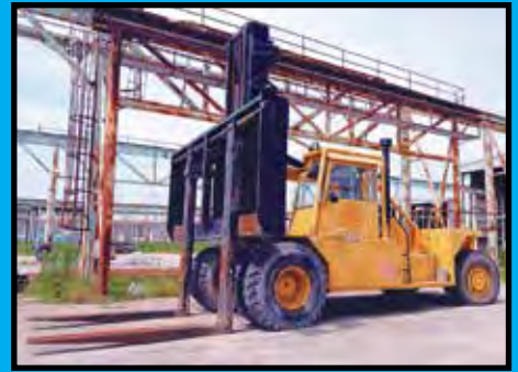
90,000 LB. CAP. TAYLOR DIESEL FORKLIFT
