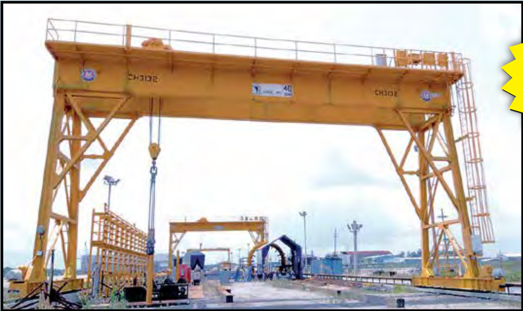
LANDEL 40 T. TRAVELING GANTRY BRIDGE CRANE
