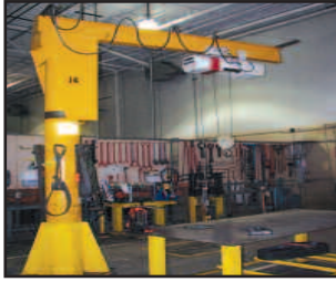
JIB CRANE WITH HOIST
