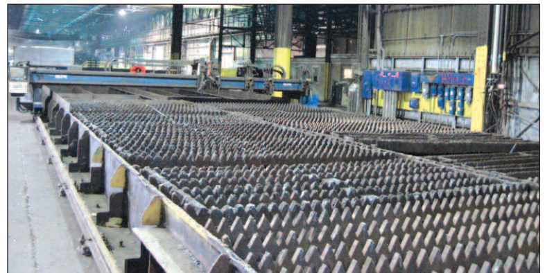
VIEW OF SECTOR PLASMA CUTTERS, WITH CLEVELAND MOTION CONTROL BURNY 10 LCD CONTROLS
