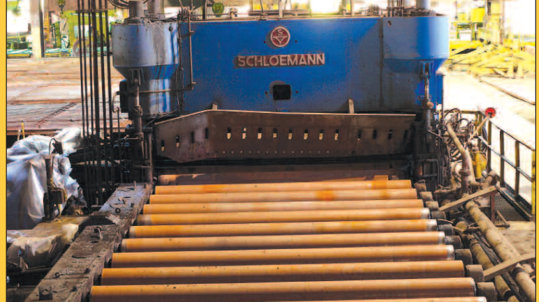
172" x 10 1/2" Dia. Schloemann 9-Roll Hot Leveler • Rebuilt 1992
