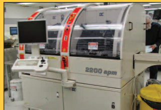
Dataconn PP52200apm Dual Gantry Fully Auto. Die Bonder. S/N 95022230878, 2001
