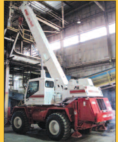
FMC Link Belt Mobile Crane
