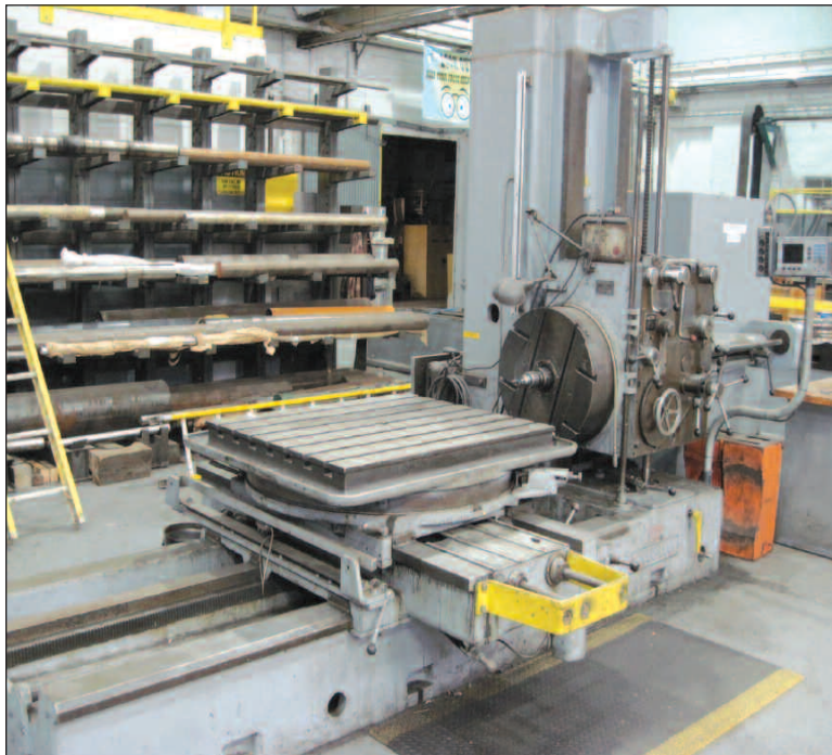
Scharman Horizontal Boring Mill
