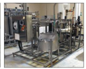
PROCESSING: Skid-Mounted 3-Tank CIP System; 2009 Skid-Mounted 1,720 GPH Pasteurizer; Skid-Mounted Flavor Injection System.
