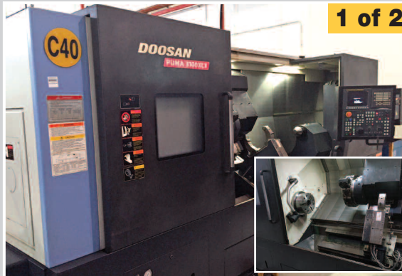
Doosan Infracore Puma 3100XLY CNC Turning Center, 84" Centers, Y-Axis, Live Tooling, Steady Rest
