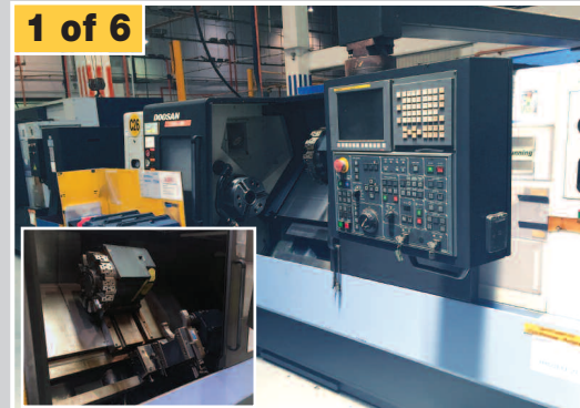
Doosan Infracore Puma 300LC CNC Turning Center 50" Centers, 4" Bar Capacity
