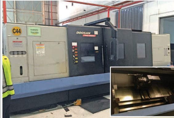
Doosan Infracore Puma 480XLM CNC Turning Center, Live Tooling, Steady Rest, 120" Centers
