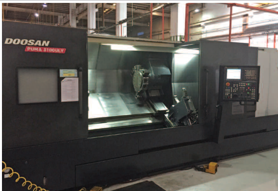
Doosan Infracore Puma 3100ULY CNC Turning Center, 120" Centers, Y-Axis, Live Tooling, Steady Rest
