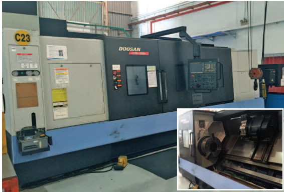
Doosan Infracore Puma 480XLD CNC Turning Center, 11" Hole Thru, 120" Centers, Dual Steady Rest, Rear Chuck
