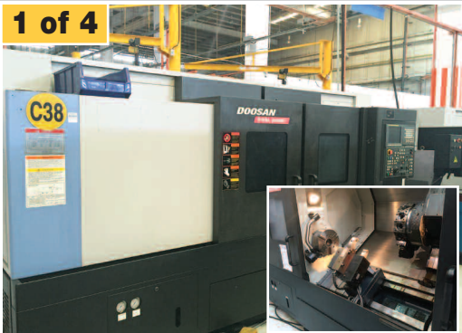
Doosan Infracore Puma 2600LY CNC Turning Center, 50" Centers, Y-Axis, Live Tooling
