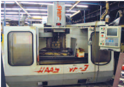
HAAS VF-3 CNC Vertical Machining Center
