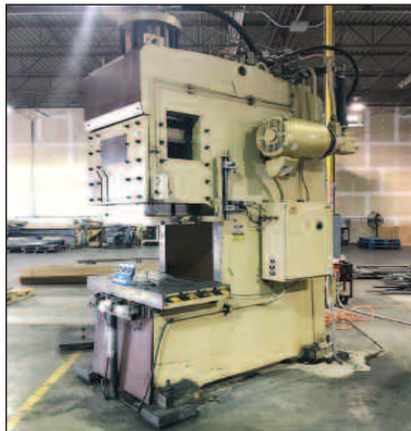
200-Ton Standard Hyd. C Frame Press
