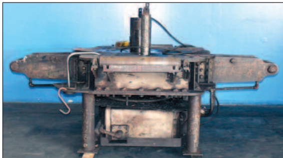
100-Ton Bull Hydraulic Camber Bender
