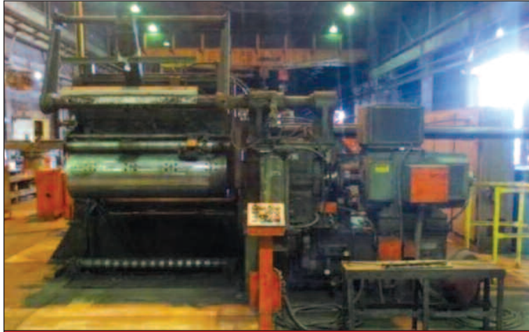
60" x 40,000 Lb. Dahlstrom Dual Head Loop Slitting Line
