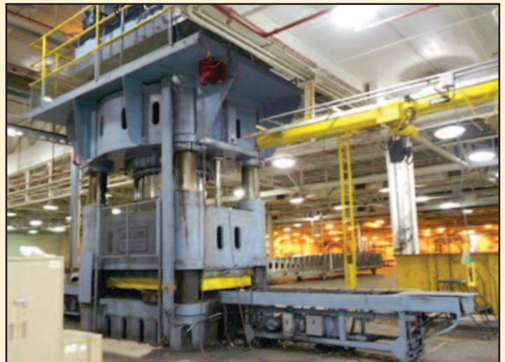
LAKE ERIE 4 POST HYD. PRESS, W/RUBBER PAD, 3,500-TON X 120" X 96"
