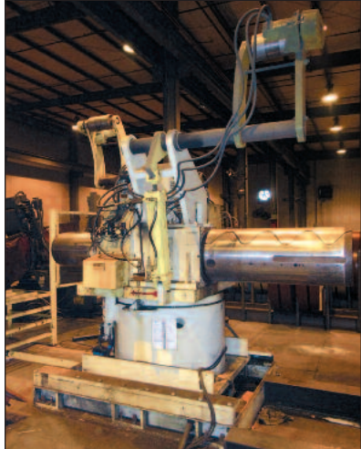
Bradbury 20k Lb. Double End Uncoiler
