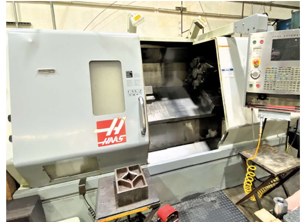
Haas SL-30T 2-Axis CNC Lathe, New 2005, 30" Swing, 17" Max Turning, 34" Max Length, 12 Pos. Turret, 3400 RPM, 3.5" Bore, 30 HP, Tailstock, Tool Setter, Haas CNC, S/N 71829
