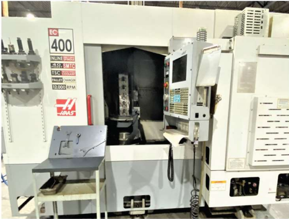
Haas EC-400 CNC 4-Axis Horizontal Machining Center, 2005, 16" x 16" Pallets, 20" X, Y, Z, 12000 RPM, 40 Taper, 40 ATC, 30 HP, Coolant Thru Spindle, Chip Conveyor, High Speed Machining, Remote Jog Handle, Visual Quick Code, Probe, S/N 51285
