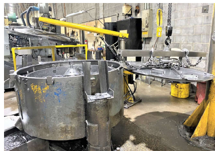
48" Tolhurst Chip Wringer with Baskets, Hoist, Jib Crane
