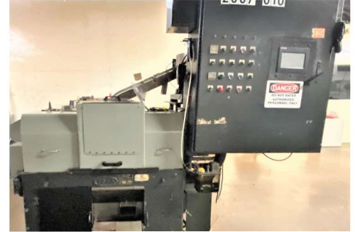
Roy Screw Slotter Model E with Feeder (2) Towa Model 10-4A Shavers
