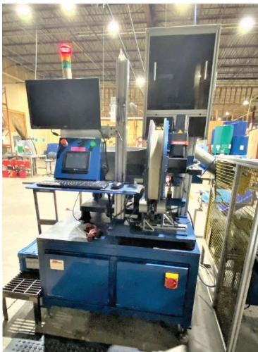
Automatic Part Inspection Machines Attica Automation Model AV-B100 Vision Inspection System, Vibratory Feed, Delta Touch Screen
