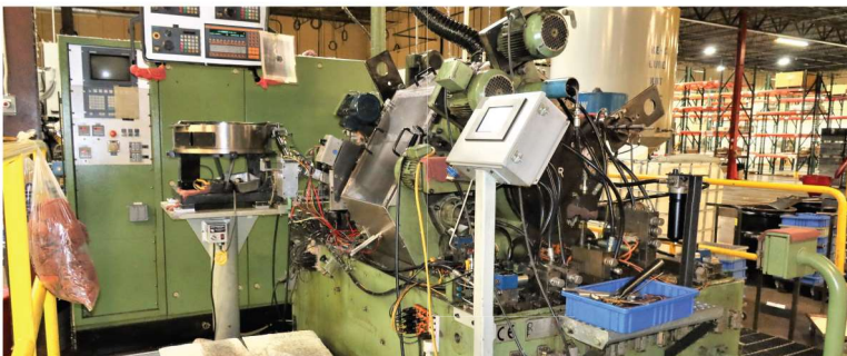
Hydromat V12 Double End Trunnion Type Rotary Transfer machine with Epic CNC Slide, S/N V12-07
