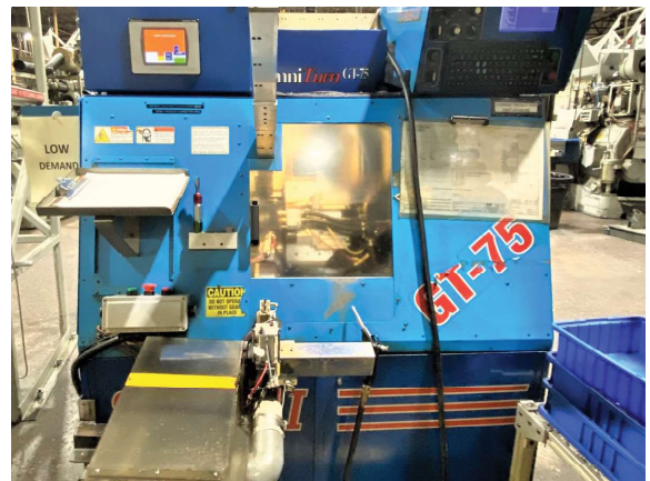
(2) Omniturn GT-75 2-Axis Gang Type CNC Lathes, 5C Collet Nose, 5 HP, 12" X, 9" Z, 4000 RPM, 6" x 14" Gang Plate, Generation 4 CNC, S/N 4691G4, 4602G4
