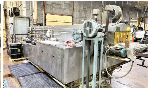
20" Wide Stainless Steel Mesh Parts Washing System, 3 Stage with Dryer, Temp. Controls
