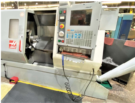
Haas SL-20 2-Axis CNC Lathe, New 2003, 23" Swing, 10.3" Max Turning, 24" Max Length, 12 Position Turret, 5000 RPM, 30 HP, 3.0" Bore, Tool Setter, Chip Auger, Haas CNC, S/N 65961
