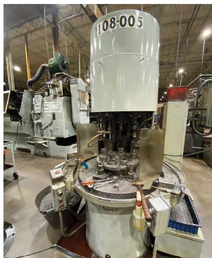
MSO Secondary Operation 3-Spindle Rotary Transfer Machine, 5C Collets
