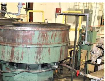
Vibratory Bowl Finishers Ultramatic 84" Diameter Bowl Vibratory Finisher, 20-25 Cubic Ft
