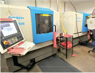
(2) Schutte WU305 5-Axis CNC Tool and Cutter Grinders, New 2002 and 2000, Universal Rotary Axis, 25000 RPM, C-Axis, 400 X, 250 Y, 250 Z, Measuring Probe, 0.0001 Resolution, Misc. Tooling, Hoffman Coolant System and Hydra Coolant System (Rebuilt 2012), Siemens 840D CNC Controls, S/N 10, 02
