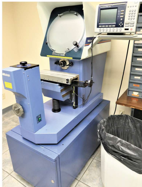
Mitutoyo PH-A14 Optical Comparator with Quadra Check
