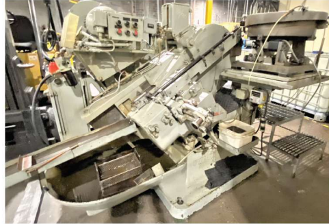
Waterbury Farrel #20 3/8" Cap. Thread Roller with Feeder
