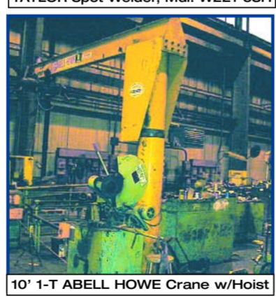
10' 1-T ABELL HOWE Crane w/Hoist
