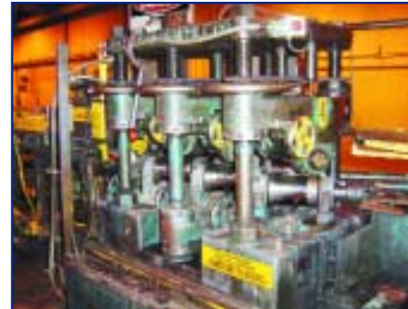
4" DIA. MACKINTOSH HEMPHILL, MDL. AN TUBE STRAIGHTENER
