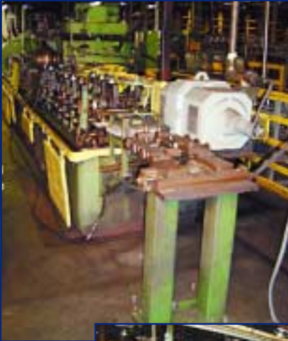
1 9/16" X .083" MIAMI WELDED STEEL TUBE MILL LINE
