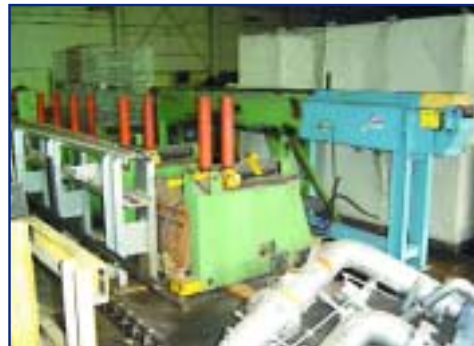
20' MAIR TUBE BUNDLING SYSTEM W/CONTROLS
