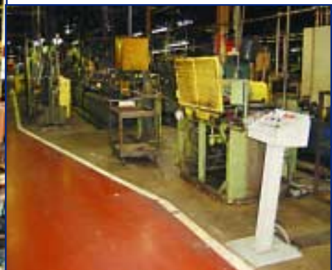
3" X .148" ABBEY ETNA WELDED STEEL TUBE MILL, MDL. 3XU
