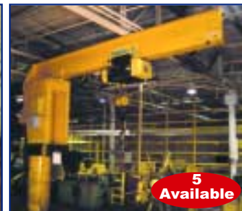
5-TON SPANCO JIB CRANE
