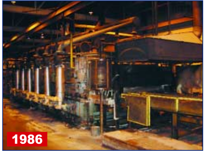
6,000 LB./HOUR SURFACE COMBUSTION GAS FIRED NORMALIZING FURNACE
